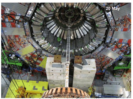
Installation of the beam pipe in CMS (minus-side).
