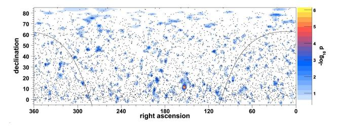
Northern hemisphere neutrino sky map in equatorial coordinates based on the IceCube data taken in 2008 (22 string detector, 276 days livetime). Each dot represents the origin of one of the 5100 detected muon neutrinos. The possible hotspot at (declination  $11^\circ$ , right ascension  $153^\circ$ ) is compatible with a statistical fluctuation of the atmospheric neutrino flux.
