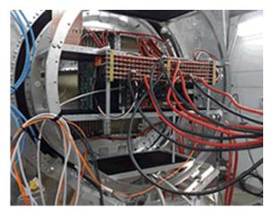
TPC being introduced in the supraconducting magnet TPC endplate.
