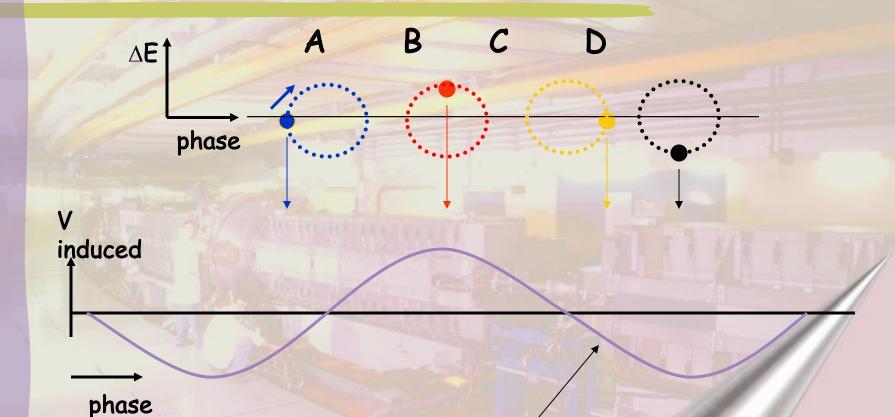
This residual voltage will accelerate B and decelerate D
