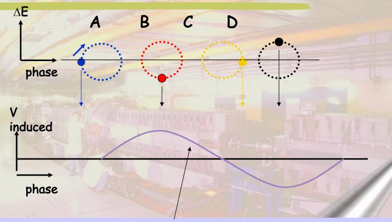
This residual voltage will accelerate B and decelerate D ⇒decrease the oscillation amplitude
