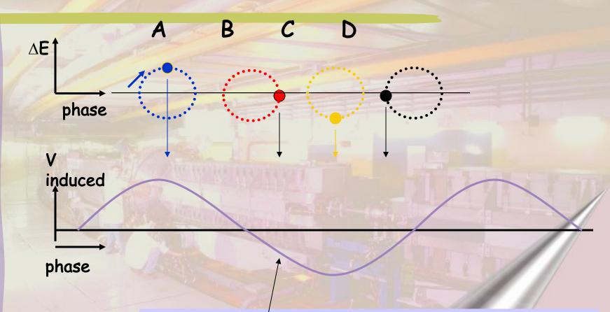
This residual voltage will accelerate A and decelerate CAgain  $\Rightarrow$  increase the oscillation amplitude
