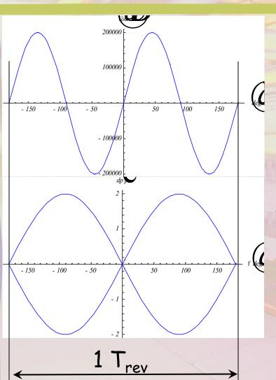
$F_{rf} = h \times F_{rev}$  Frequency of cavity voltage Harmonic number
