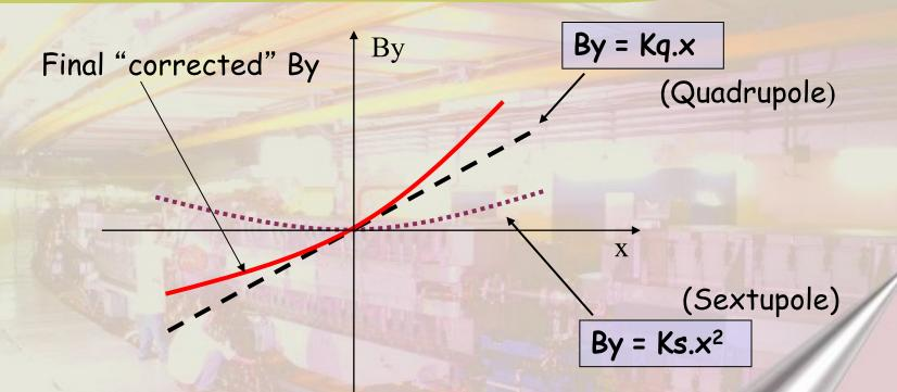
Vertical magnetic field versus horizontal displacement in a quadrupole and a sextupole.
