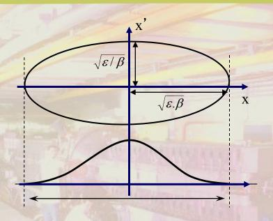
✓ The projection of the ellipse on the x-axis gives the Physical transverse beam size.
