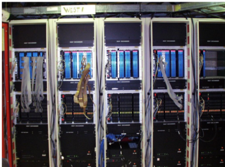
CDF L1&L2 Calorimeter Triggers: 12 9U Crates
