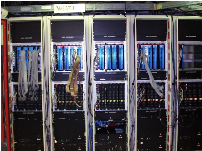
CDF L1&L2 Calorimeter Triggers: 12 9U Crates
