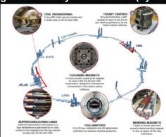
New IR-quads Nb<sub>3</sub>Sn (inner triplets) New 11 T Nb<sub>2</sub>Sn (short) dipoles Collimation upgrade Cryogenics upgrade **Crab Cavities** Cold powering Machine protection Civil engineering
