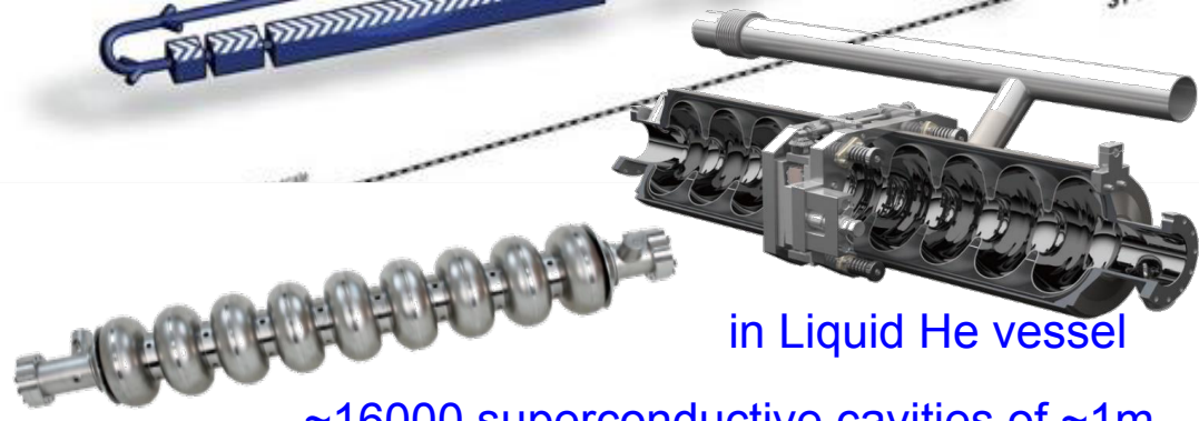
~16000 superconductive cavities of ~1m
