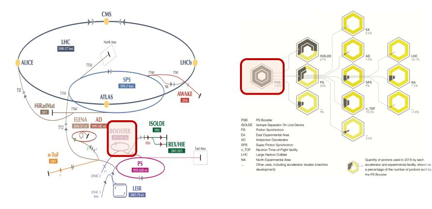
The CERN accelerator complex and the LHC – protons from Booster only <0.1% to LHC
