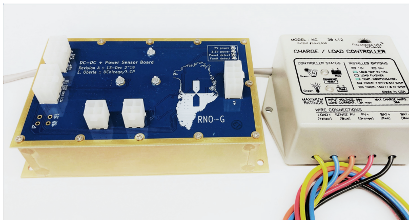
Figure 21. The station solar charge controller and high-efficiency DC-DC board for RNO-G.
