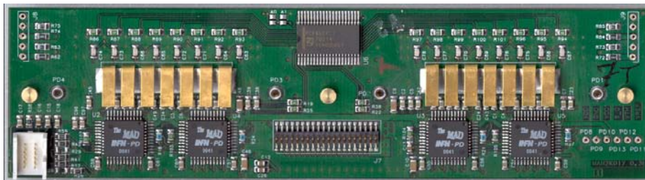
Figure 7.15: Front-end board (FEB).
