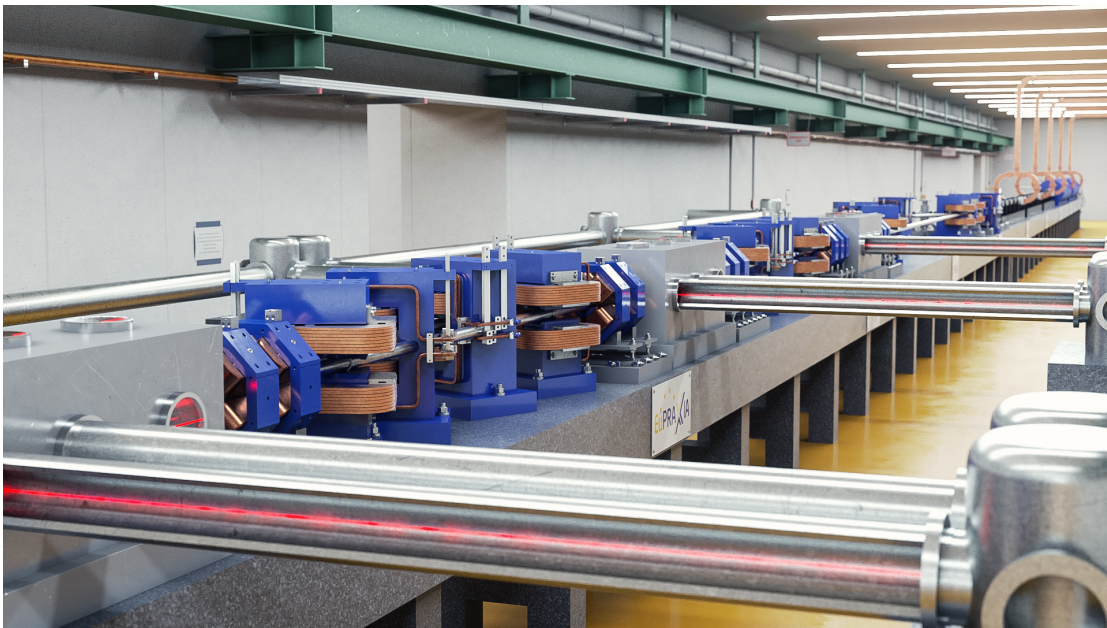
Rendering of the two-stage, very-low-energy-spread plasma accelerator developed for the EuPRAXIA facility. The open tubes show the paths of the laser pulses (red lines) that drive the plasma wakefields in the vacuum boxes.
