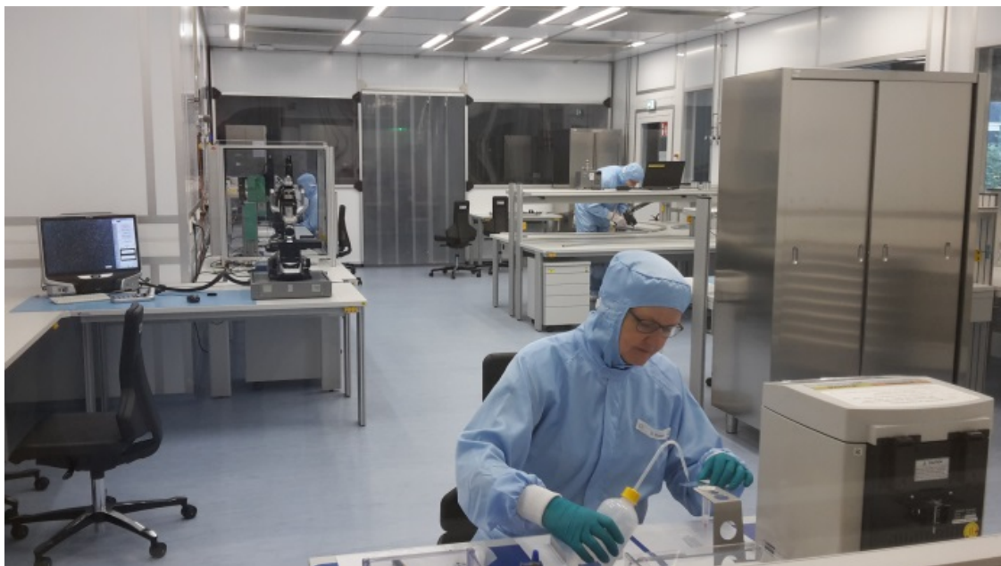
View of the CMS area of the DAF cleanroom at DESY, with microscopes and automated module assembly system. All major devices have been installed and are being commissioned.
