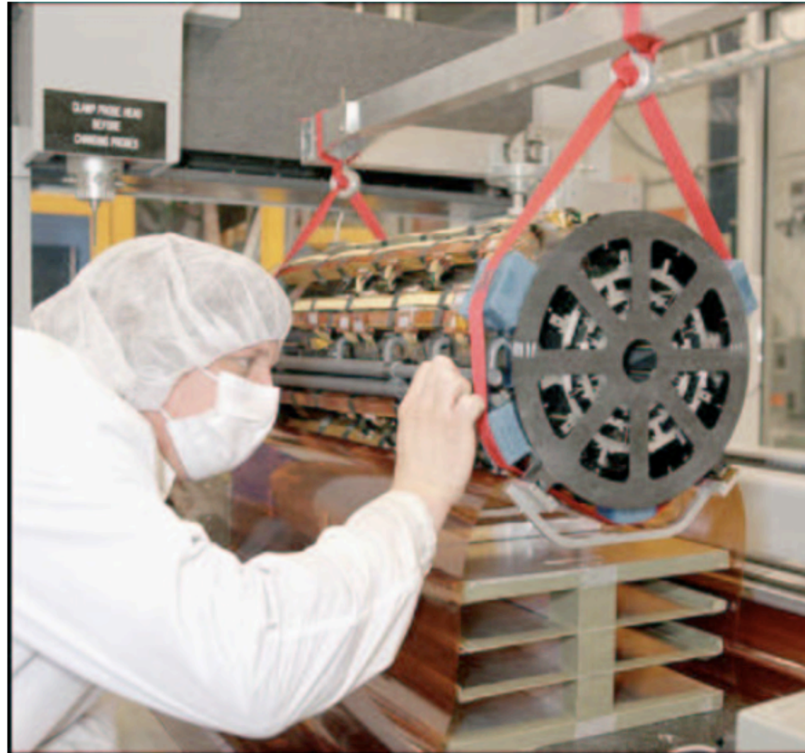
New Vertex Detector for CDF (or D0?). 1 Million strips
