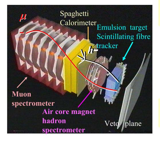
Hadron Sign and momentum Air-core magnet hadron spectrometer  $\Delta p/p = \sqrt{(0.035 \cdot p(GeV/c) + 0.22^2)}$
