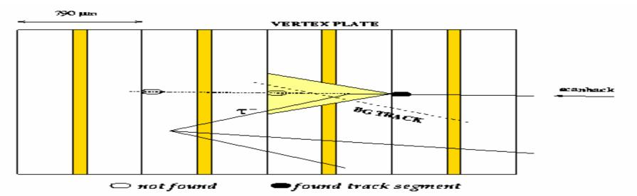
100  $\mu m$  most upstream of the vertex plate are searched for all track segments in a cone of width  $\propto 1/P$
